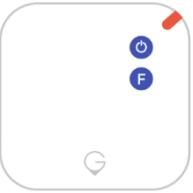
Press and hold Power and F button for 2seconds. LED flashes in RED and BLUE.
